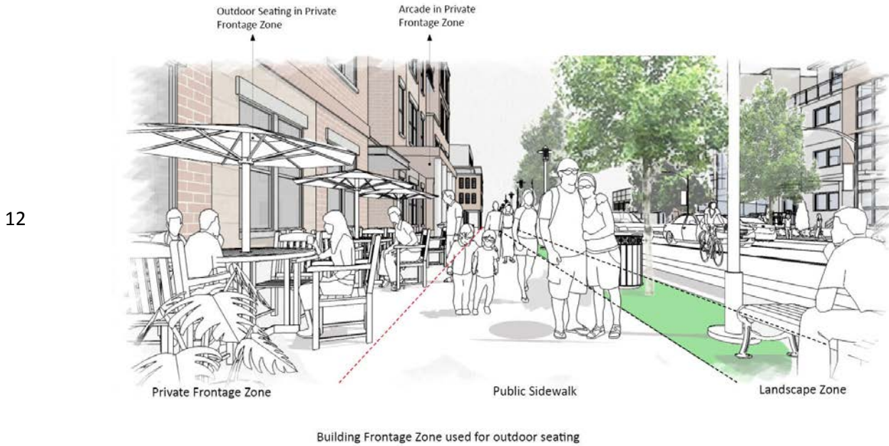
10 Figure V - 8: Examples of Building Frontage Zone Activity 11
