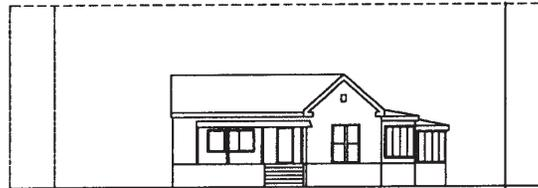
*The overall order of the building elevation relative to the side lot setbacks and maximum allowable height (dashed lines).*
